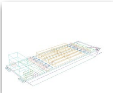
The top deck holds the reverse osmosis units
